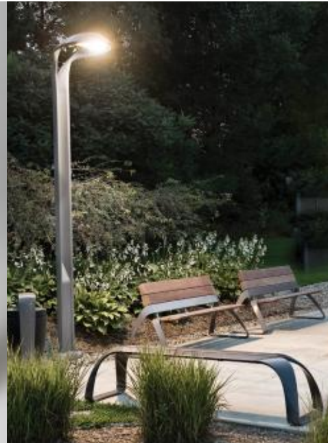
Landscape Forms, Inc. Hi-glo Pedestrian Light Structure: Cast aluminum; pole is aluminum extrusion. 12'-6" high. Exceeds IESNA DG-5 lighting standards.
