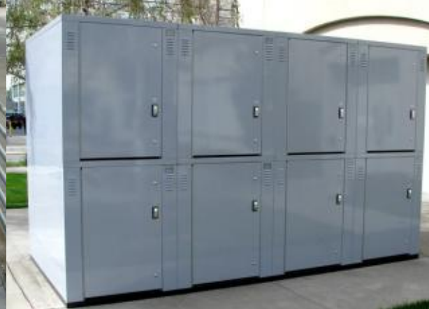
durabikelocker.com Standard DL2 locker Solid or perforated galvanized steel, with finish options. 39" w x 48" h x 75" l; internal divider for two bikes. Can be stacked double height, in rows.
